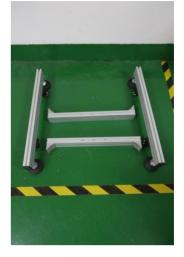
3. Place the nuts into the aluminum profile and begin mounting the base. 4.Base Installed.
