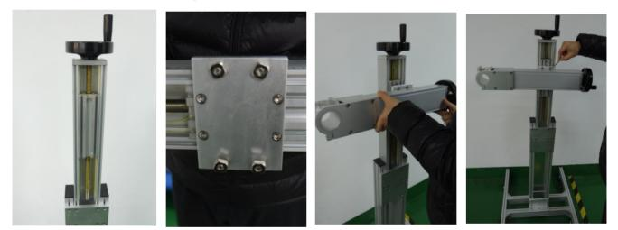
7. Find the corresponding screws of bracket and start mounting the laser bracket.
