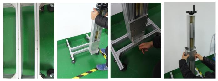
6. Take out the bracket horizontal bar, remove the nuts and put into the longitudinal slide and install the bracket horizontally.
