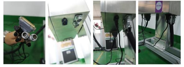
10. Connect the device power cable, and turn on screen button->laser button. (Except the emergency stop button, the button can be disconnected under emergency circumstances)
