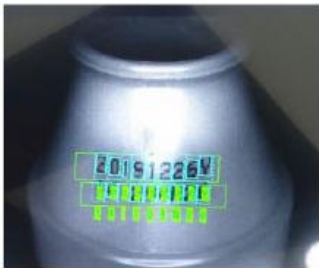
OCR character inspection for coding on the bottle
